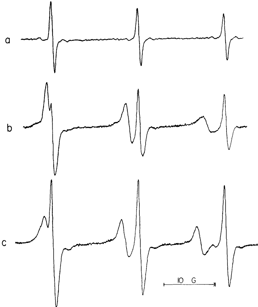
Fig. 8. 35 GHz ESR spectra of di- t -butyl nitroxide in (a) 0.1 M potassium phosphate buffer, pH 6.5, (b) aqueous suspension of membranes of the microsomal fraction, (c) aqueous suspension of myelin. All spectra were recorded at room temperature, but not necessarily with the same spectrometer gain
